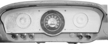
2. Remove these four screws to separate the bezel from the gauges.
